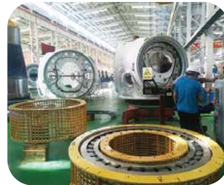
Heating bearing inner&outer ring for mounting
