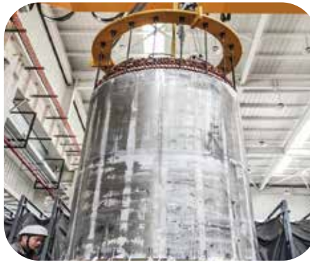
Heating motor housing for dismounting
