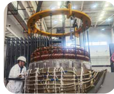
Heating motor housing for dismounting
