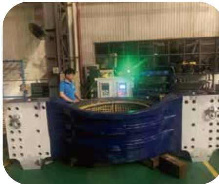
Heating bearing housing for mounting
